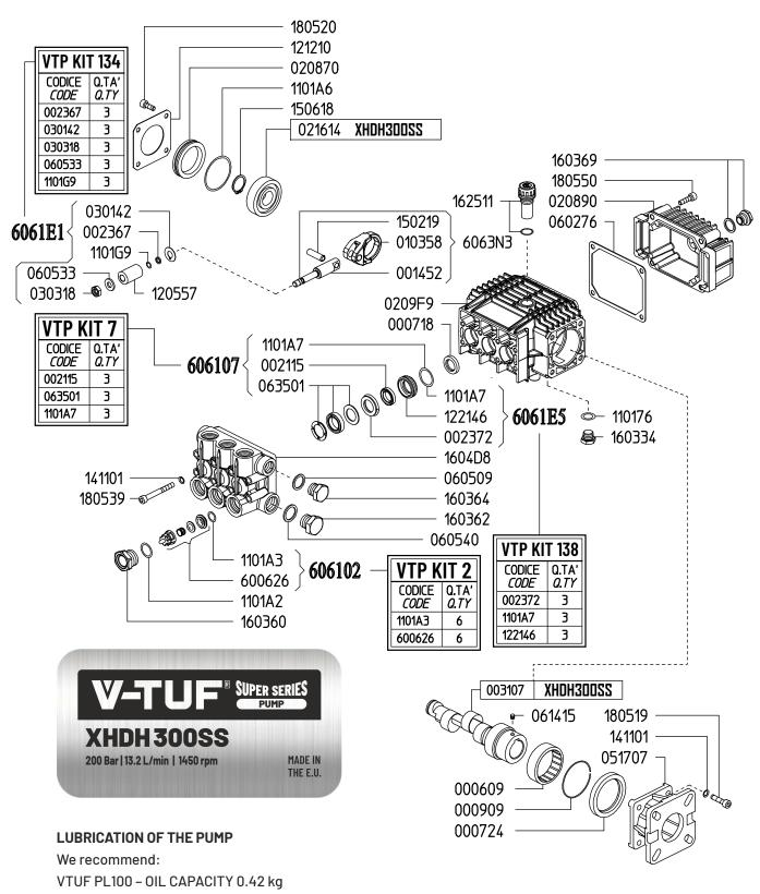
You should change the oil after the first 50 hours of use, and after each subsequent 500 hours of operation.
