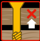
Partially Threaded Stops The Timber Jacking
