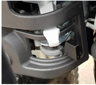
Fig5: Warm start or trouble start position - Engine Fuel tap lever (black) to the right and choke lever (grey) in centre position. Don't forget to move this choke lever immediately to the right (off position) when the engine starts running
